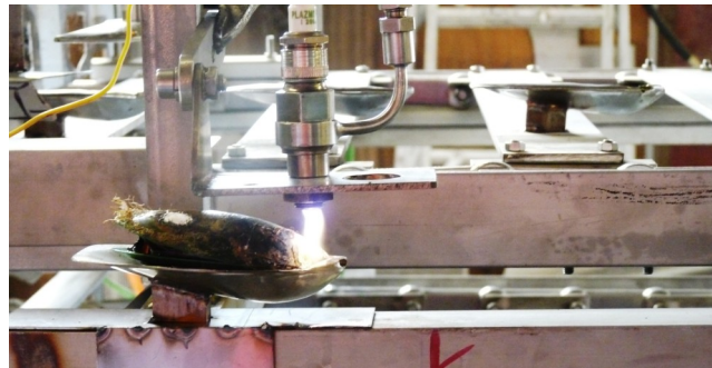
Fig. 2. Non-thermal torch for mussel opening
