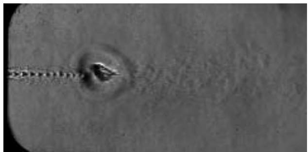
Fig. 2. Schlieren image of M3 combustion chamber after laser pulse
