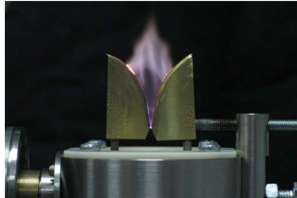
Fig. 1. Principle of gliding arc operation and time-integrated photograph of discharge luminosity ( R_b = 10 \text{ k}\Omega , C_c = 300 \text{ pF} , V_0 = 3 \text{ kV} , R_{sh} = 1 \text{ }\Omega ).
