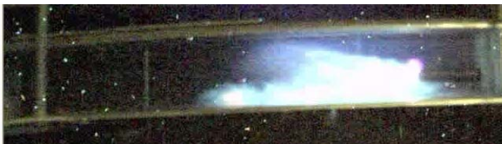
Fig. 5. Initial moment of the gas-air mixture ignition under the combined impact of the external electric field and the electron beam
