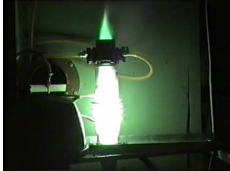
Fig. 8. Nitrogen combined operation mode of hybrid (DC + RF) plasma torches
