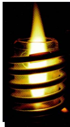
Fig.1. Plasma induction heating 1 – inductor, 2 – plasma, 3 – quartz tube
