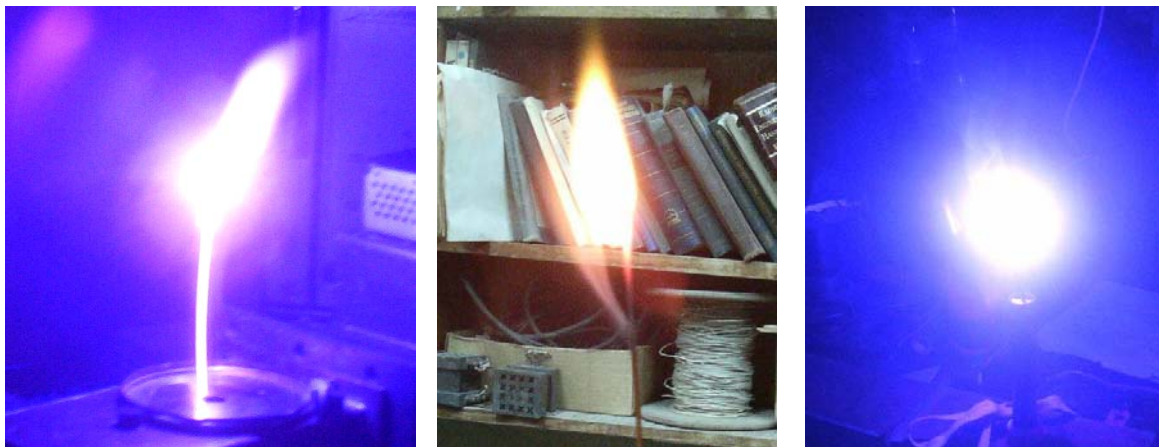
Fig. 2. The discharge initiated at the end portion of the single-wire Goubau line.
