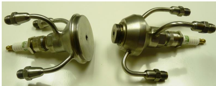
Fig.2. PFN modifications with the cross flow channels.
