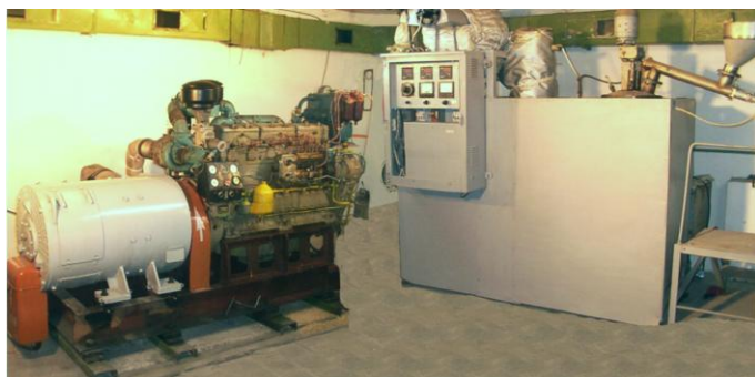
Fig.1. An experimental facility for thermoplastic waste processing into artificial fuels
