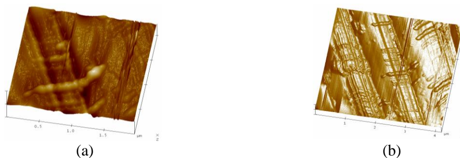
Fig.3. (a) Before water-plasma pretreatment. (b) After water-plasma pretreatment. ( Z=100 nm/div)
