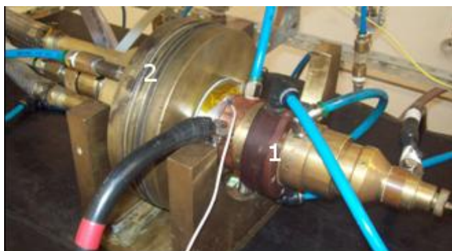
Fig.1. Experimental system. Plasma torch (1) acopled with quenching chamber (2)
