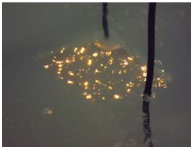
Fig.1. Plasma discharge phenomena in PEO
