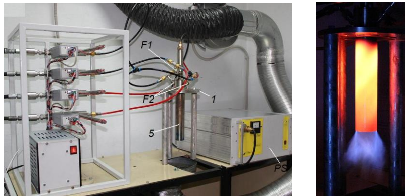
Fig.3. Photograph of the torch flame generator and the combustion chamber with the torch flame at its exit
