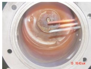
Fig.3. Double counter flow at combustion of propane (0.5 g/s propane, air mass rate 38.5 g/s)
