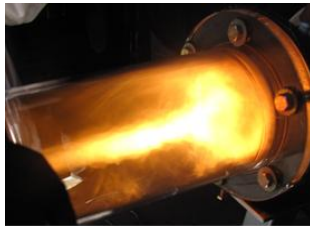
Fig.1. Combustion of 1.6 g/s kerosene at the air mass rates 36 g/s with umbrella-like combustion zone. One can see spiral tracks of liquid fuel from left to the right
